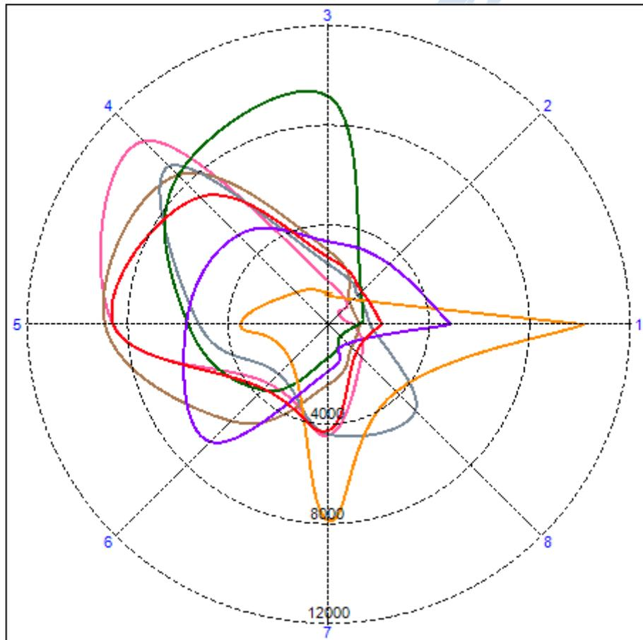
Figure 1. 8 channel polar plot showing a visual representation of the EMG patterns for 7 movements. Each coloured shape represents a movement and each axis is a channel. Activity on each of the channels are plotted for each movement and lines are connected to get an idea of the 'shape' of the movement in feature space. By visual appraisal it can be determined how to make EMG patterns more separate.
