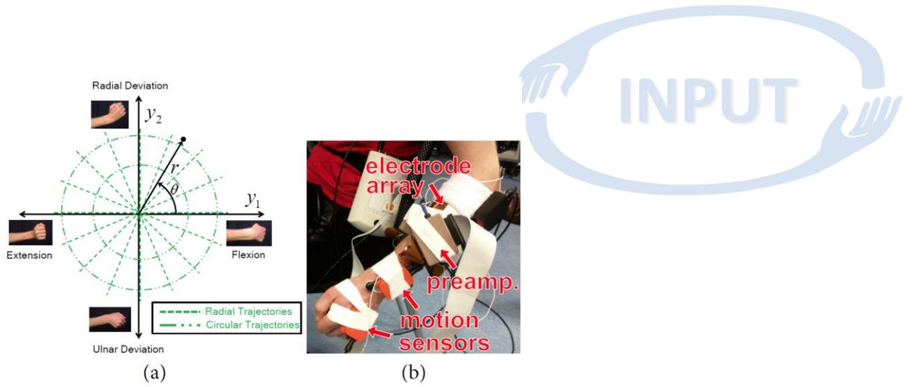
Fig. 1: (a): Visualization of the trajectories within the 2D space spanned by the two DOFs. (b): Experimental Setup involving EMG acquisition with an electrode array and motion capturing system.
