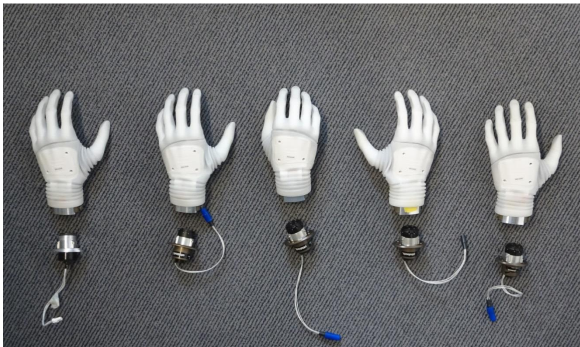
Figure 1: The 5 Michelangelo prostheses available for INPUT, including active wrist flexion prototypes and wrist rotations.
