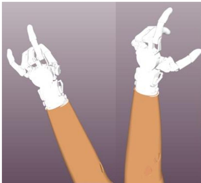
**Figure 6: Unlike the real prosthesis, the virtual can also move individual fingers only**
