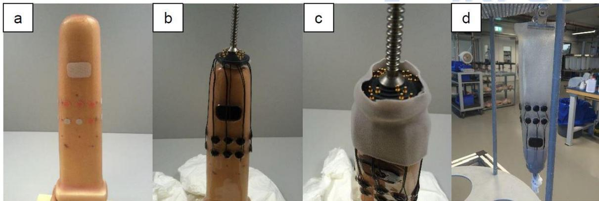
**Figure 2. Improved liner mould with electrode dummy positions (a), placed connector with connected wires (b), distal connector with fabric cover to fix wires (c), preparation for coating (d).**
