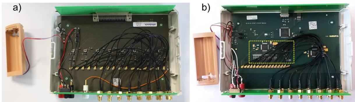
**Figure 3. Comparison between the desktop EMG acquisition system. a) Previous desktop amplifier based on discrete components (AMYO project). b) Desktop amplifier based on analog front-end. The image shows a desktop setup for 16 bipolar channels; only the marked zone is required for 8 bipolar channels.**
