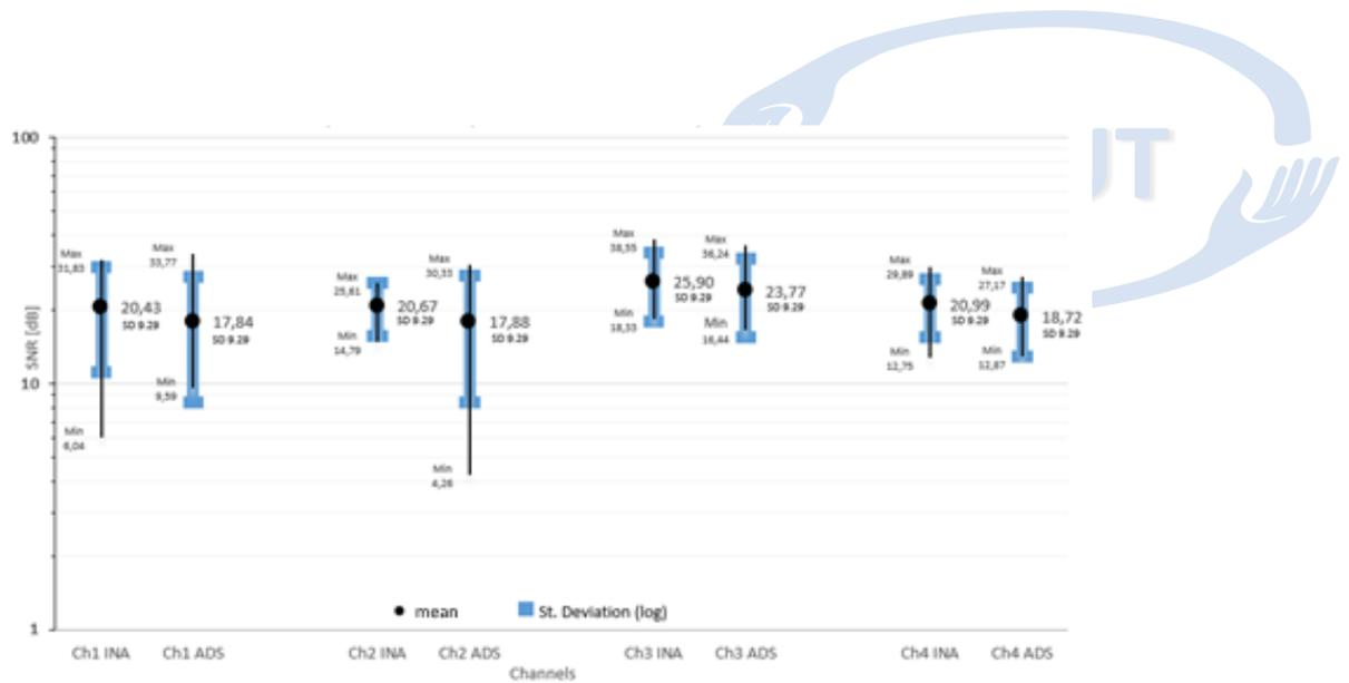
**Figure 4. Comparison between previous desktop amplifier based on discrete components (INA) and the developed signal acquisition system based on an analog front-end (ADS). Four bipolar EMG channels were recorded.**
