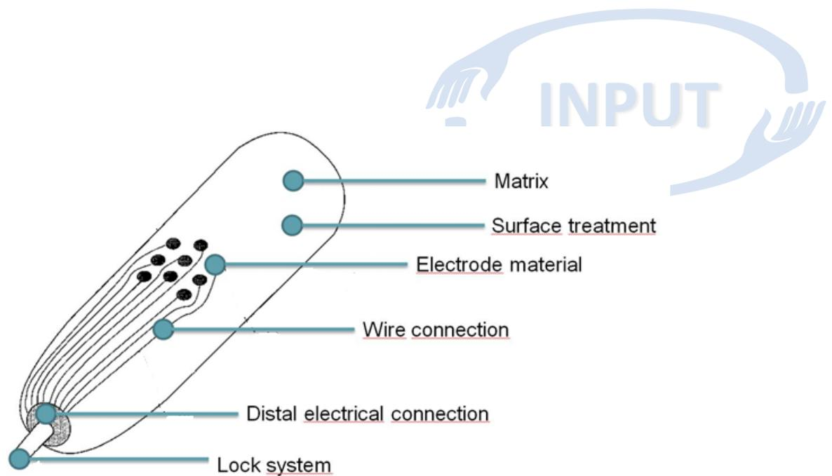
**Figure 1. Schematic overview of the parts of the electrode liner.**
